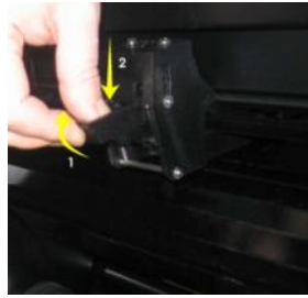
FIG 5-1 LIFTING THE PINCH ROLLER
