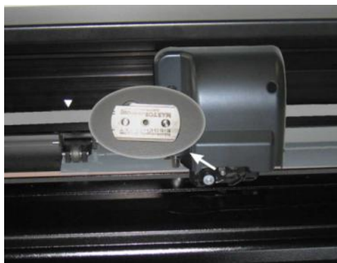
FIG 1-35 RAZOR BLADE FOR AUTOMATIC SEPARATION OF MEDIA
