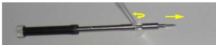
FIG 1-24 REMOVING KNIFE FROM THE TANGENTIAL KNIFE HOLDER
