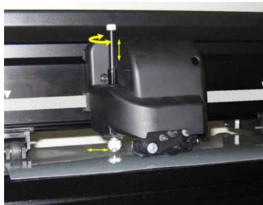
FIG 1-26 INSERTING THE TANGENTIAL KNIFE HOLDER
