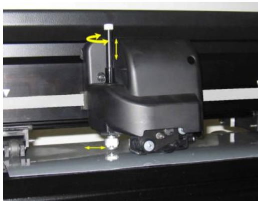
FIG 1-23 REMOVING THE TANGENTIAL KNIFE HOLDER
