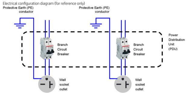
NOTE: The Power Distribution Unit (PDU) must be rated to meet the power requirements of the printer, and shall be in accordance with the Electrical Code requirements of the local jurisdiction of the country where the equipment is installed.
