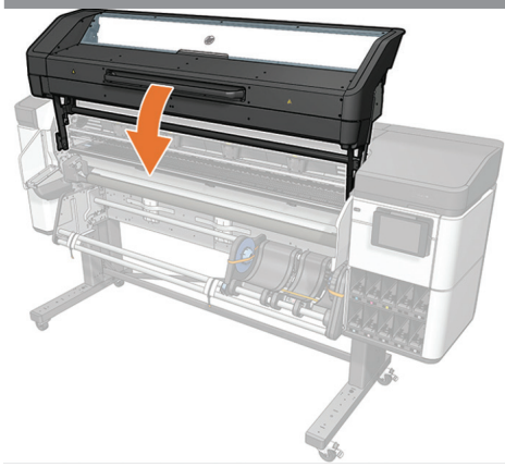
Lower down the curing module.
